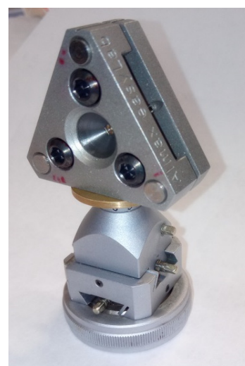
The high-pressure cell for the room-temperature XRD experiments, mounted on a diffractometer holder adjusted for the cell.
