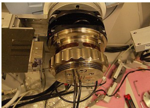
Left: Panalytical MPD mounted with high temperature chamber. Right: PXRD patterns for Ti-NT system during heating in air.. Measured with the presented diffractometer and adapted from T. Vaclavů. Et al., J Therm Anal Calorim 128 , 779–785 (2017).
